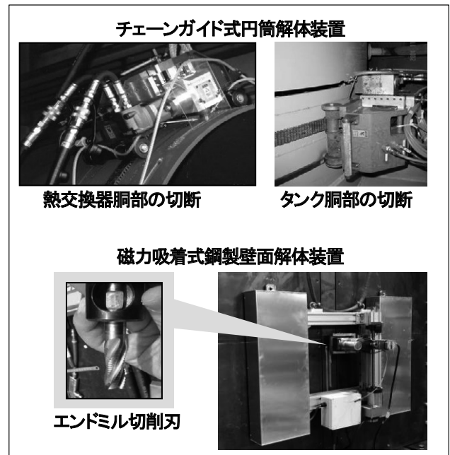
Fig.14 Cutting devices using milling cutter
